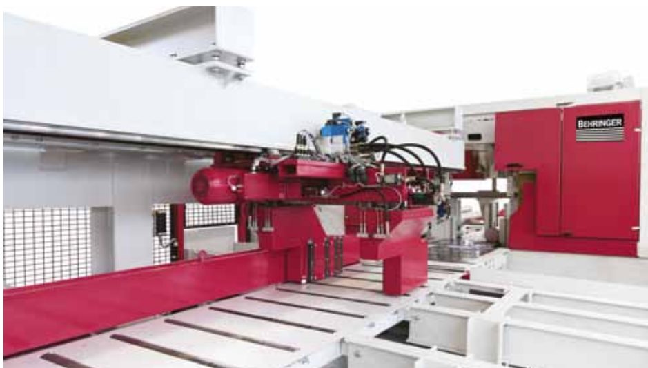
Voss is establishing a dedicated cutting centre to cut bars and heavy material into individual lengths. Photo: Timo Lutz Team für Industriefotografie.
