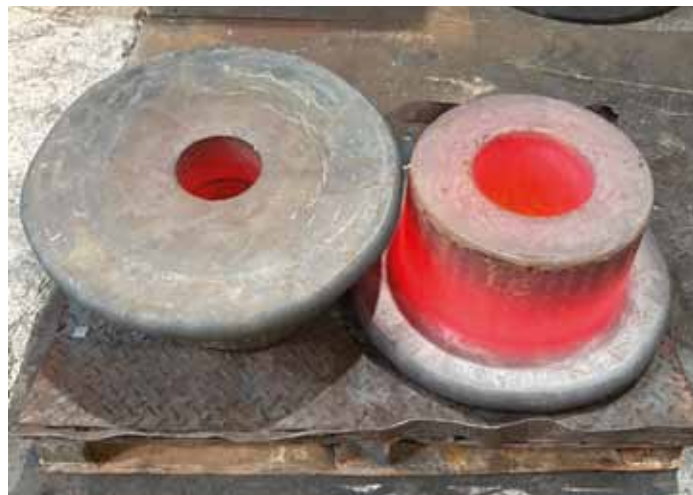
Components forged close to contour in the nickel-based alloy Alloy 601/UNS N06601.
