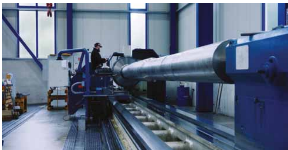
The Torni Tacchi HD3-120H CNC lathe enables machining of components up to 26 meters in length and 1,540 mm in diameter.
