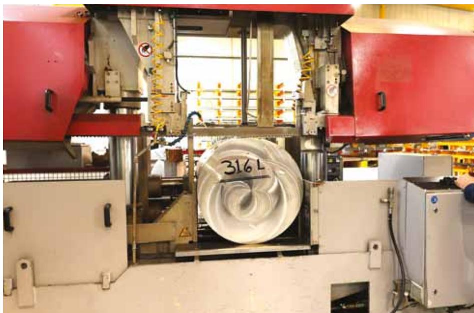
*Sawing a 764 mm diameter piece of 316L steel*
