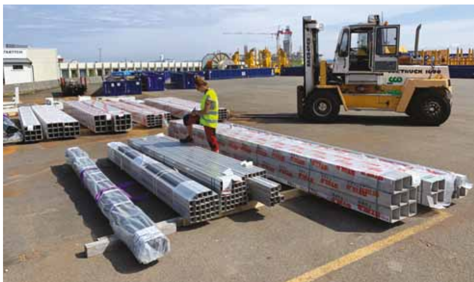
Sverdrup supplied over 2,000 meters of lean duplex hollow structural sections, plates and hot rolled angle bars.
