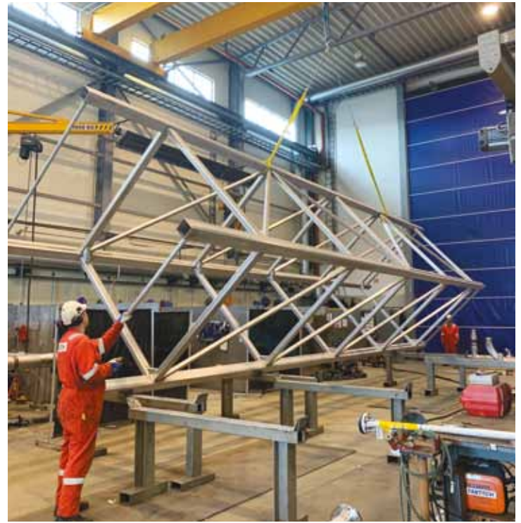
The lightweight lean duplex bridge resulted in reduced costs for handling, fabrication, welding and logistics and material compared to carbon steel structures.
