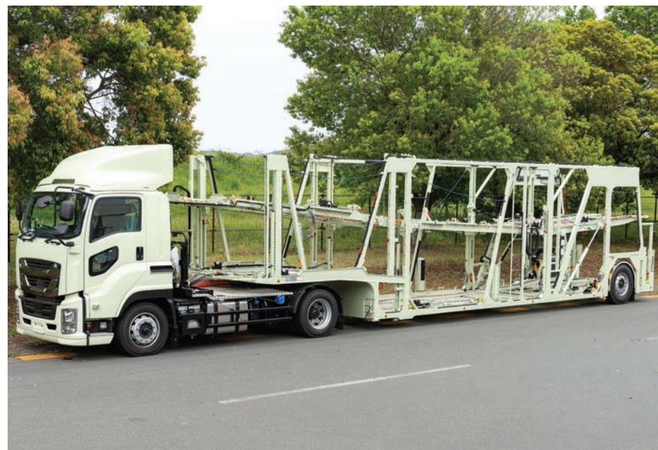
A stainless steel truck frame reduces life-cycle costs and weight, allowing car carriers to carry more vehicles.
