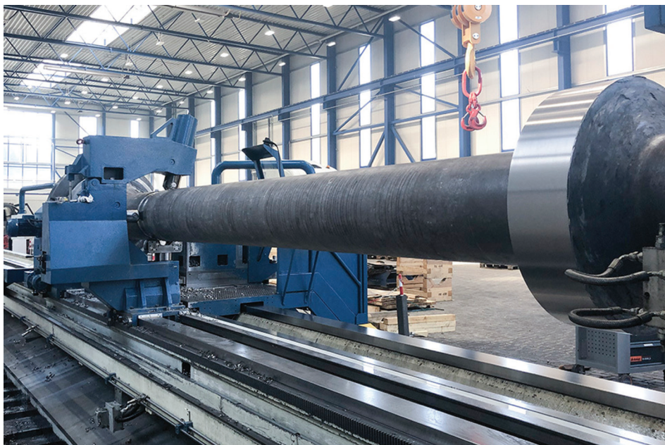
The company's new Torni Tacchi (HD3-120H CNC) lathe can machine components with a length of up to 26 meters and a diameter of 1,540 mm.
