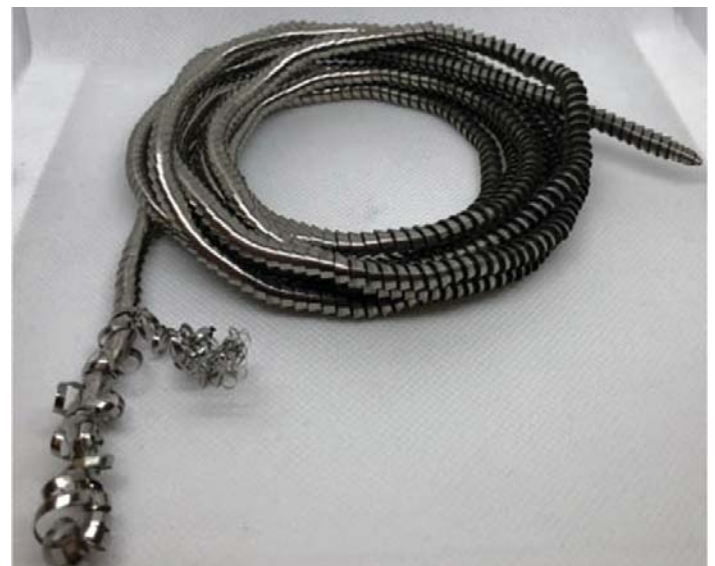
An endless chip could wind itself around the workpiece, tool, or machine chuck and can pose a hazard to the machine or your safety. It can help to change the direction of rotation and the approach angle of cut. © Image source: ARNO
