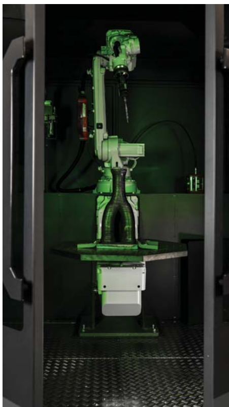
The M1 system, a fully integrated solution for WAAM printing
