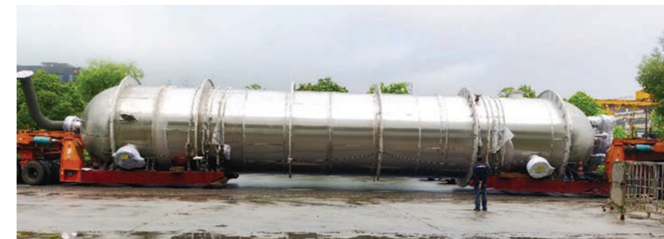
Polycrystalline silicon manufacturing devices made of NASH38X(UNS N08120). Photo courtesy of Jiangsu Sunpower Heat Exchanger & Pressure Vessel Co., Ltd.
