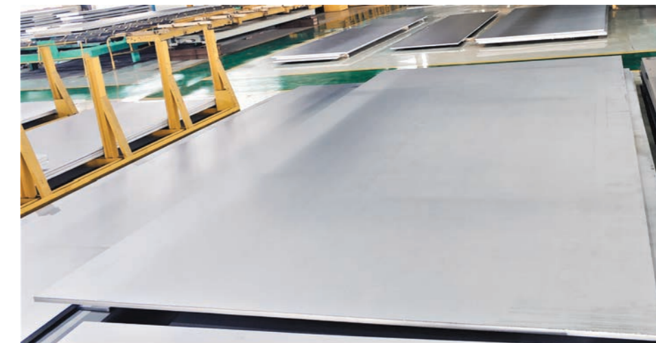
3270mm wide plates of alloy NAS800T (UNS N08811).
