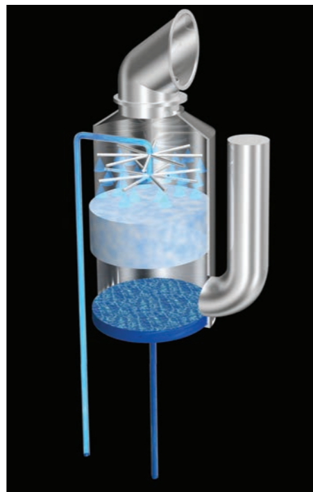
A SOx marine scrubber.
