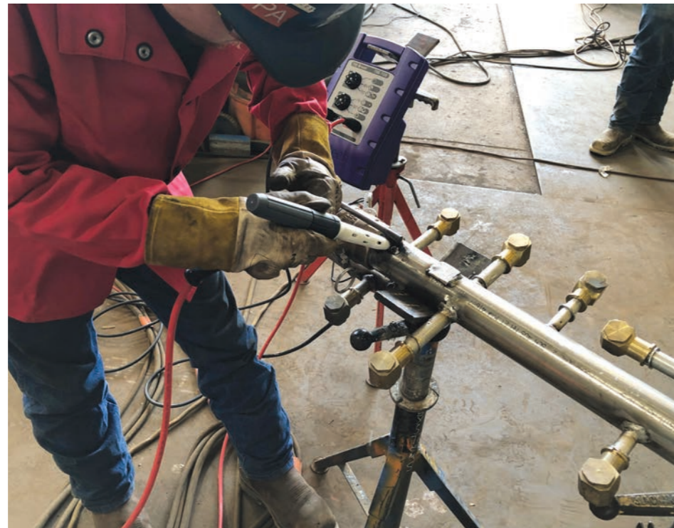
Utilising the TIG Brush means valuable welders can spend more time welding and less time cleaning.
