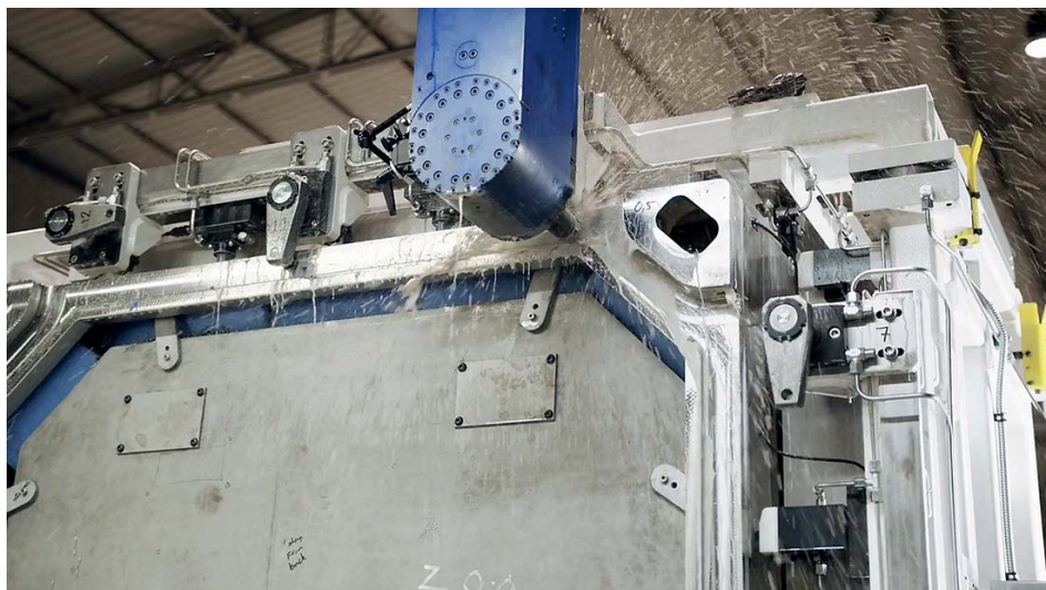
Close-up of machining in progress, showing the way in which the hydraulically actuated swing clamps sequentially rotate out of the path of the oncoming milling cutter.
