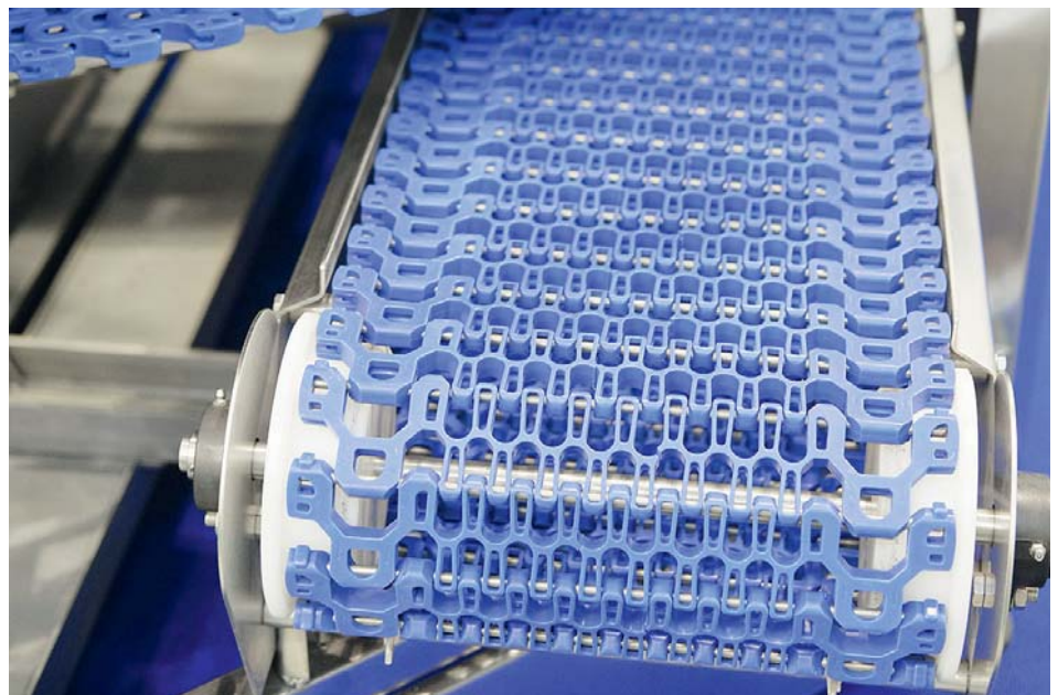
Plastic conveyor belt used in the food industry produced with metal additives to avoid foreign object contamination.
