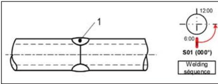
Figure 5: Welding sequence.
