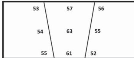
Figure 7: Ferrite content ASTM E562 at 12h.
