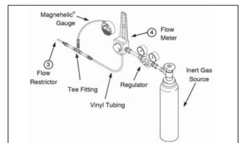
Figure 3: SWS internal purge pressure kit Swagelok.
