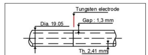
Figure 4: Welding preparation.
