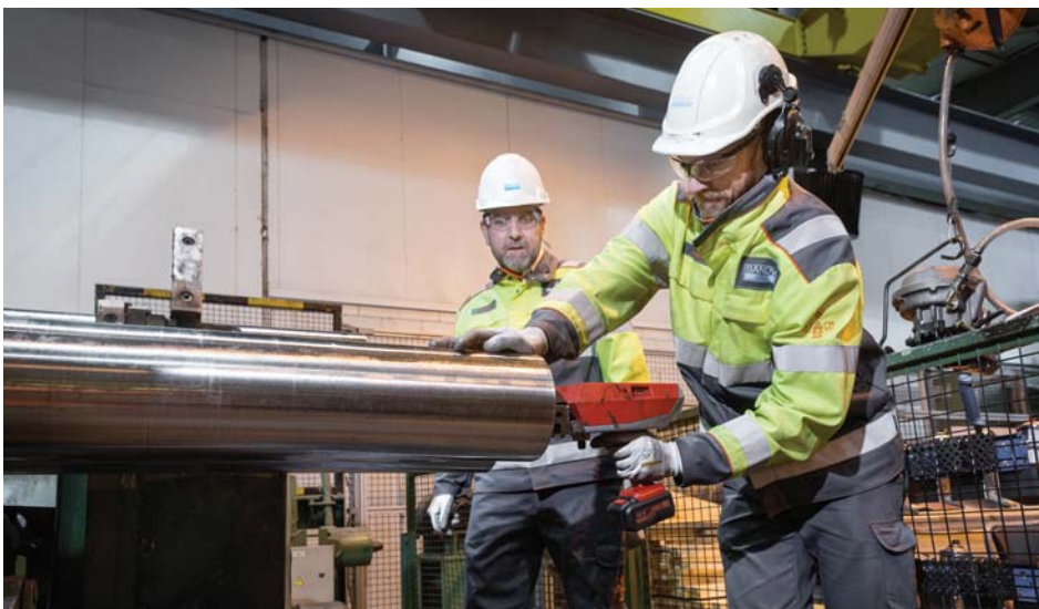
Visual inspection and marking for identification are carried out on every bar.
