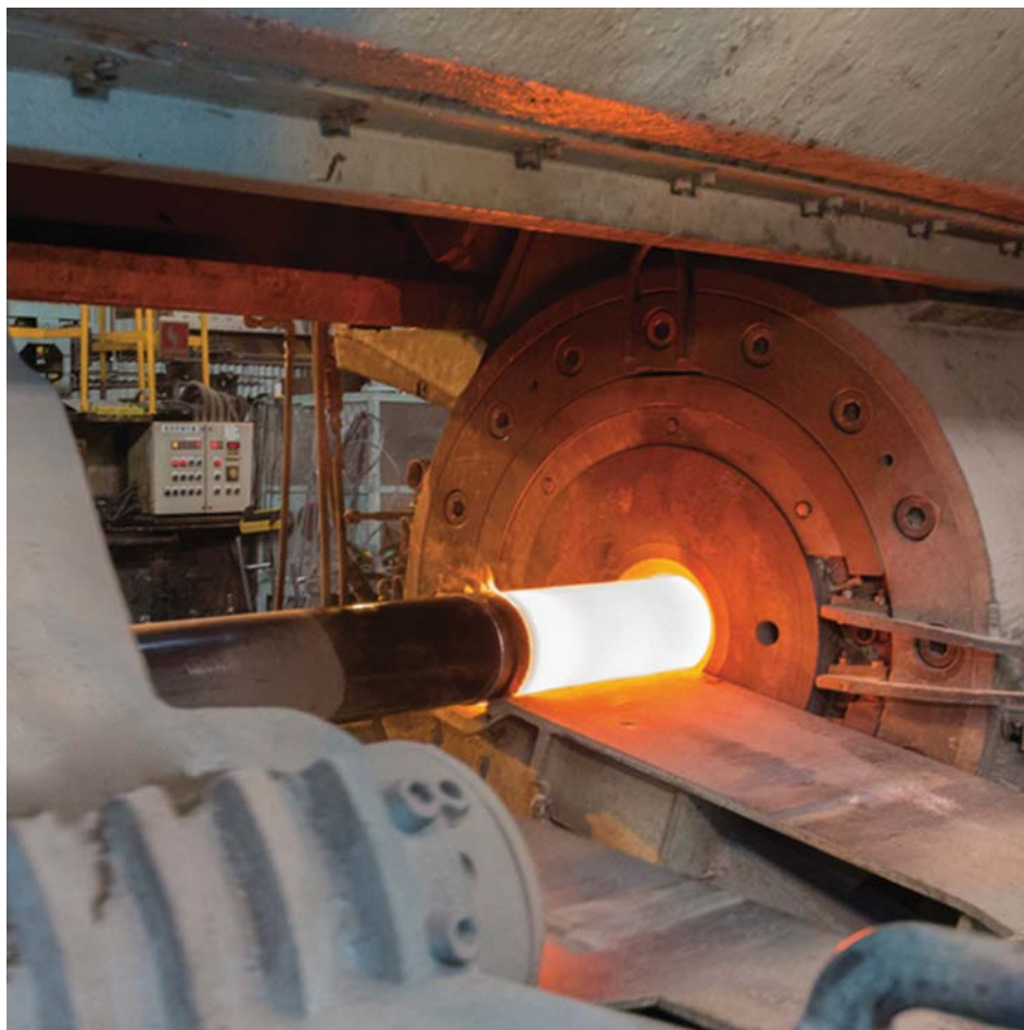
The company has produced seamless stainless steel pipes and tubes using the hot extrusion process for over 60 years.
