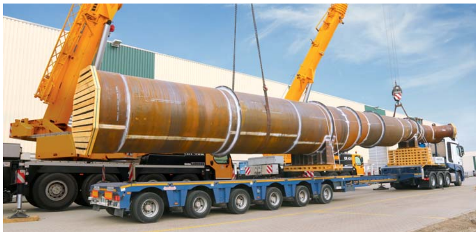
Clad mega spool for refinery having a weight of 18 tons, a diameter of 2 meters and a total length of 22 meters.
