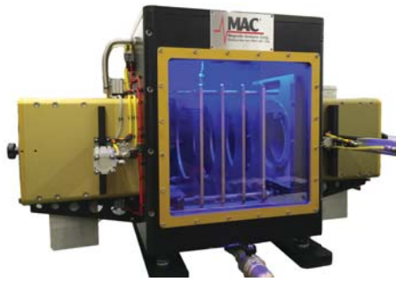
Test Head for MAC's first Ultrasonic Phased Array tester, installed at a bar mill in Italy.
