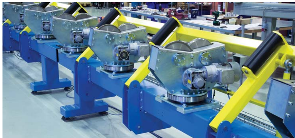
A custom designed helical spinning conveyor system ensures accuracy as tubes are fed into MAC's new APC (Automatic Pitch Control) full body ultrasonic tube tester.
