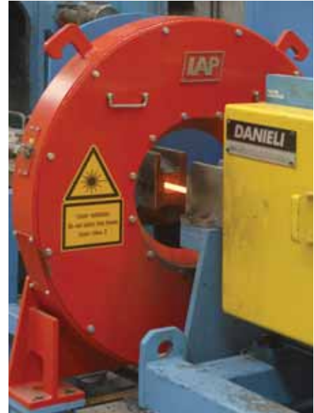
Close-up of laser gauge.
