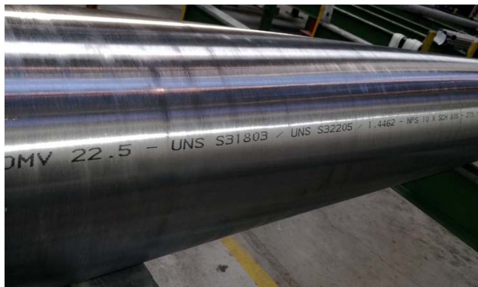
10 inch NB pipe in duplex manufactured with the Montbard/France extrusion press
