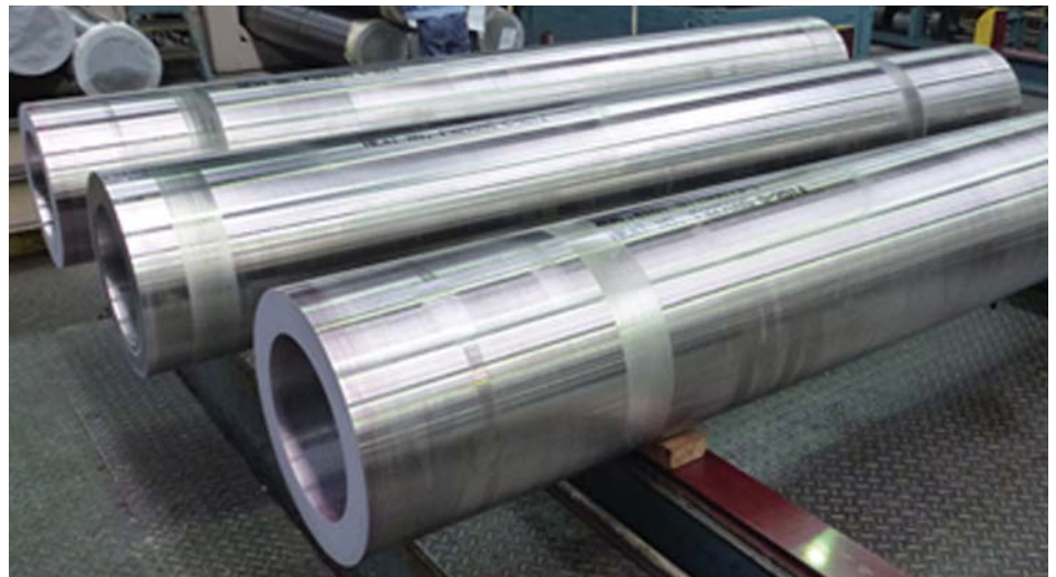
NSSMC's grade HR 6W is an important product for the extremely high temperatures that are produced in modern coal-fired power generation. Ni alloy tubes
