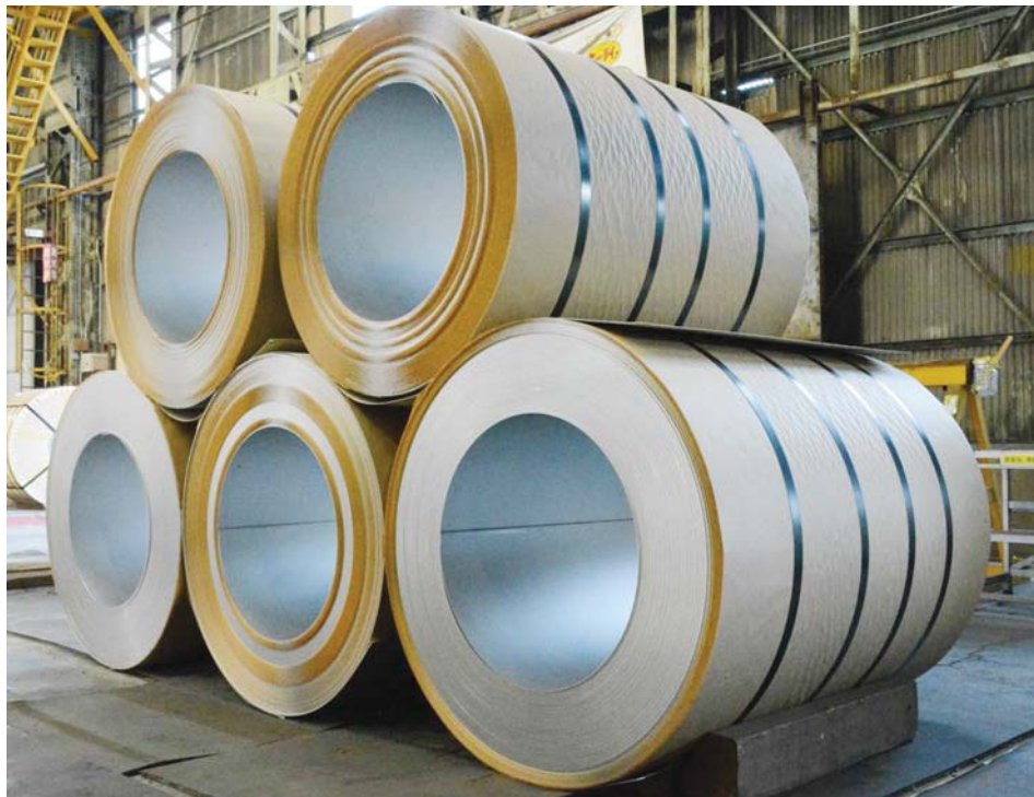
The company produces NAS NW276 (UNS N10276) hot rolled 4-foot wide coils and is increasing production of 5-foot wide cold-rolled sheets.
