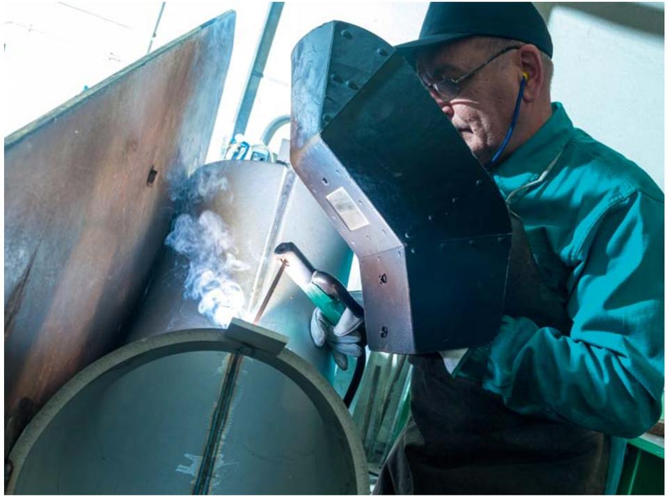
16” elbow in duplex 31803 welded at Petrol Raccord
