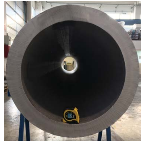
Heavy wall welded elbows and welded pipes (w.t. 50mm).
