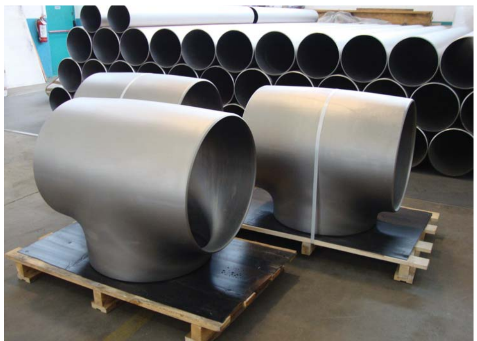
The company now has the capacity to produce hot formed heavy wall fittings like tees (up to 24”) and elbows.
