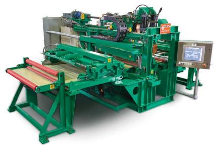
The NB Overlap welder is most commonly found on lines such as paint, tension leveling, etc.
