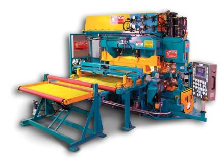
The QM Series Seam Welders produce high quality welds that are generally no more than 10% thicker than the parent material.
