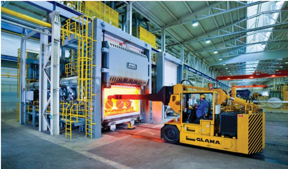
The Böhler car bottom furnace for the rotary forging process.
