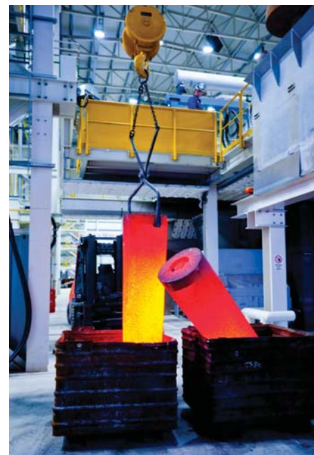
Böhler ingots produced in an induction furnace.
