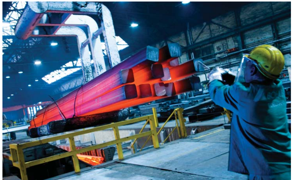
The Böhler rolled bar material and blooming mill in action.
