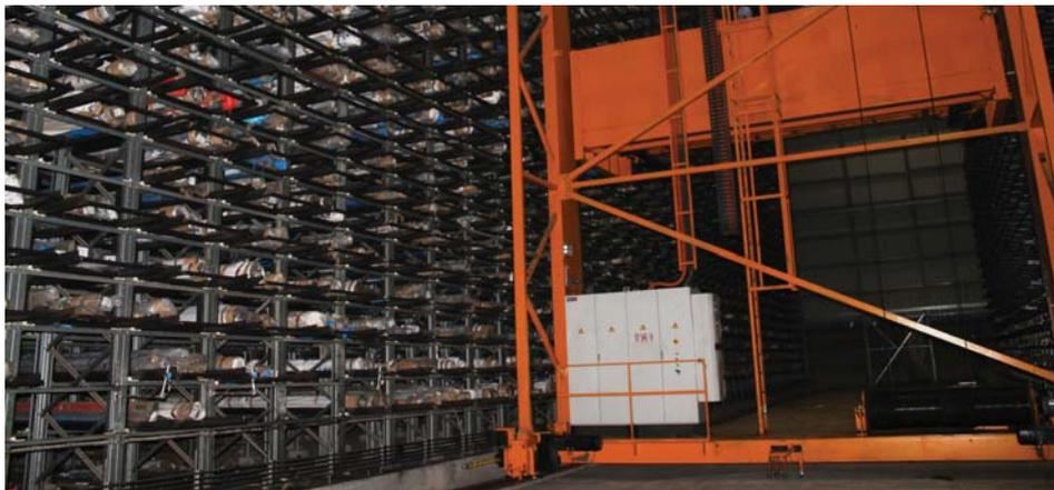
*The SRM plant's FeHR cassette rack system - also known as a honeycomb warehousing system - enables rapid storage and retrieval of bars at the touch of a button.*
