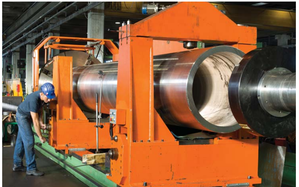
Tubacex Group wide range in seamless stainless tubes has increased through IBF's trepanning technology, equipment and expertise.
