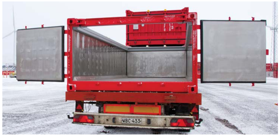
Finnish company, Lant Group Cargo Solutions, chose Outokumpu’s high-chromium austenitic grade Supra 316plus for their new special cargo containers which will be used for transporting corrosive and sharp bulk materials.
