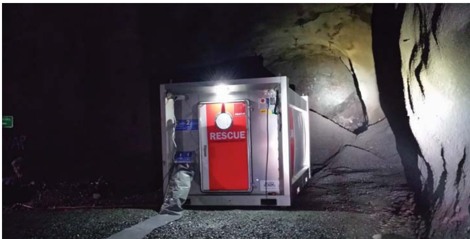
HEAT-IT Oy from Finland selected Outokumpu's new high chromium ferritic stainless steel Core 4622 as the material for their RESPETRA rescue chamber. The RESPETRA rescue chamber is a stainless steel cabin used in underground mines. It provides shield and protection for miners for example in case of fire for as long as for four days. Core 4622 is technically very suitable for the rescue chamber due to its good combination of strength and toughness and can thus handle pressure relief well. The walls of the rescue chamber are curved to provide protection against pressure and gases. Photo courtesy of HEAT-IT.
