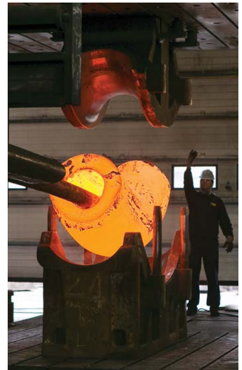
Manufacturing of a large diameter and thickness elbow at Petrol Raccord.
