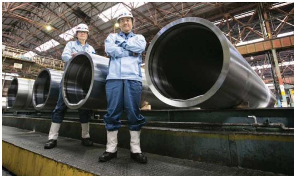
HR6W pipes manufactured for advanced USC boilers.
