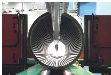
Automatic forming of welded pipes.
