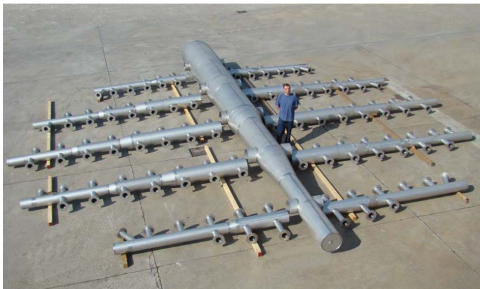
Absorber spray bank in 254 SMO.
