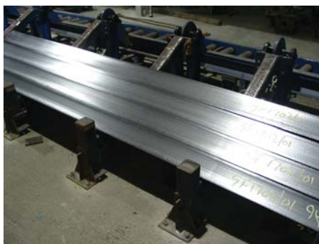
Nickel alloy 718 flat bars after forging.
