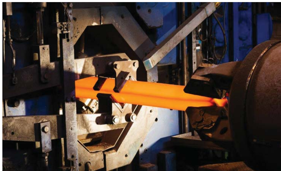
GFM SX26 producing a flat bar in nickel alloy 718 for gate valves.
