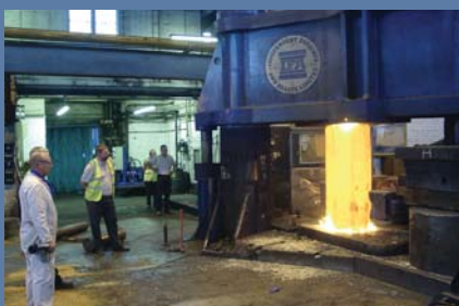
Alloy 690 ingot being upset forged for the Nuclear industry.
