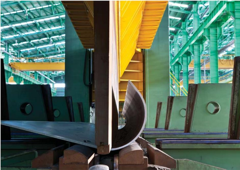
A press bending machine at the company's SunCheon Plant for large diameter pipes.
