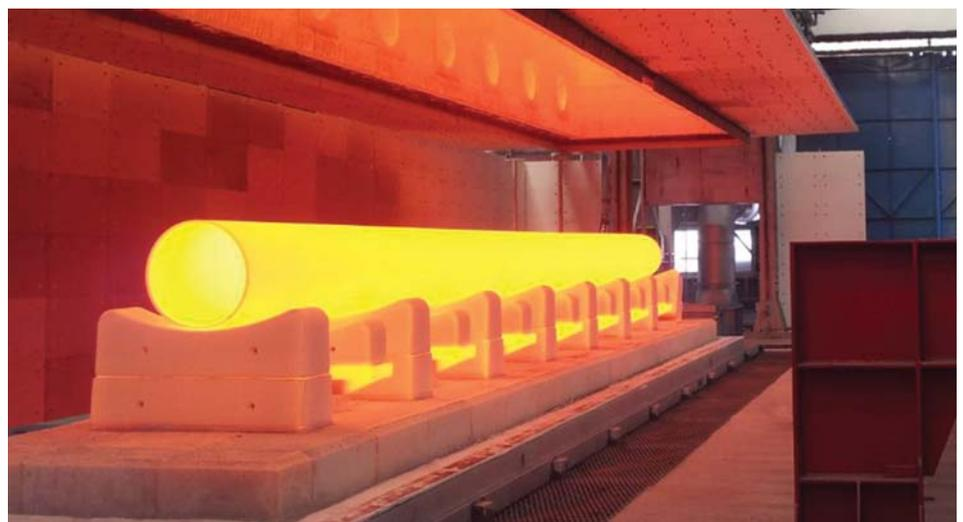
Stainless steel pipe undergoing heat treatment in the company’s Suncheon plant.
