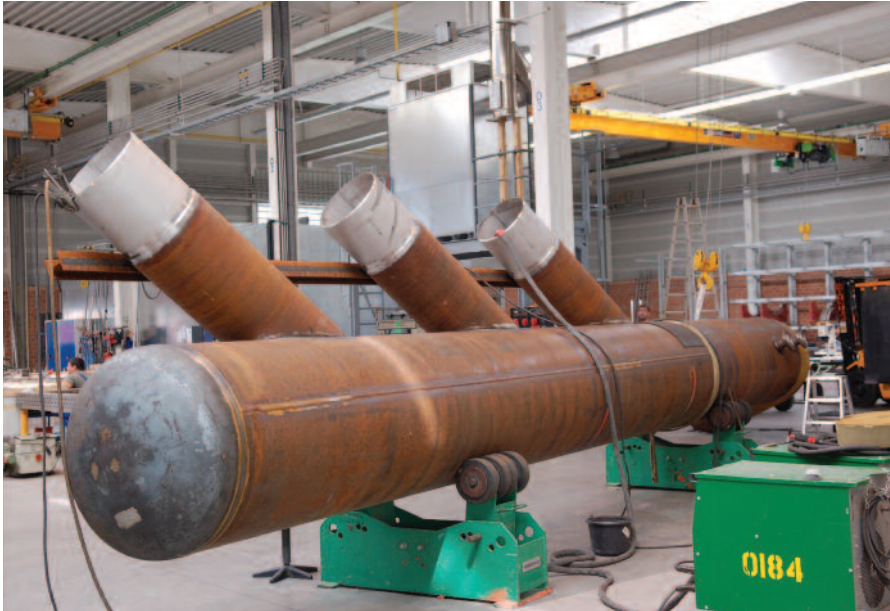
The know-how: Processing of corrosion resistant steels and clad steels into components ready for installation using appropriate material-specific welding techniques.
