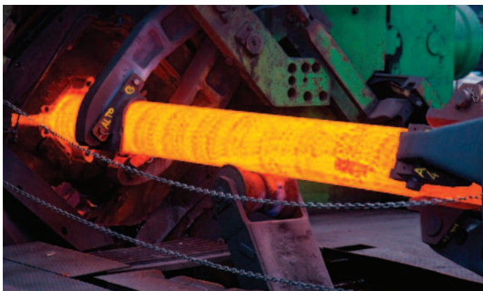
The policy at Italfond has always been to invest in modern equipment, such as this rotary forging machine.
