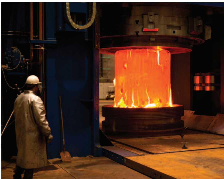
A 8.000 ton hydraulic press.
