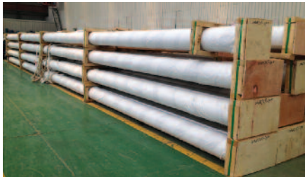
API 5L CRA welded line pipe LC80-2507 ready for delivery for Shell offshore project.
