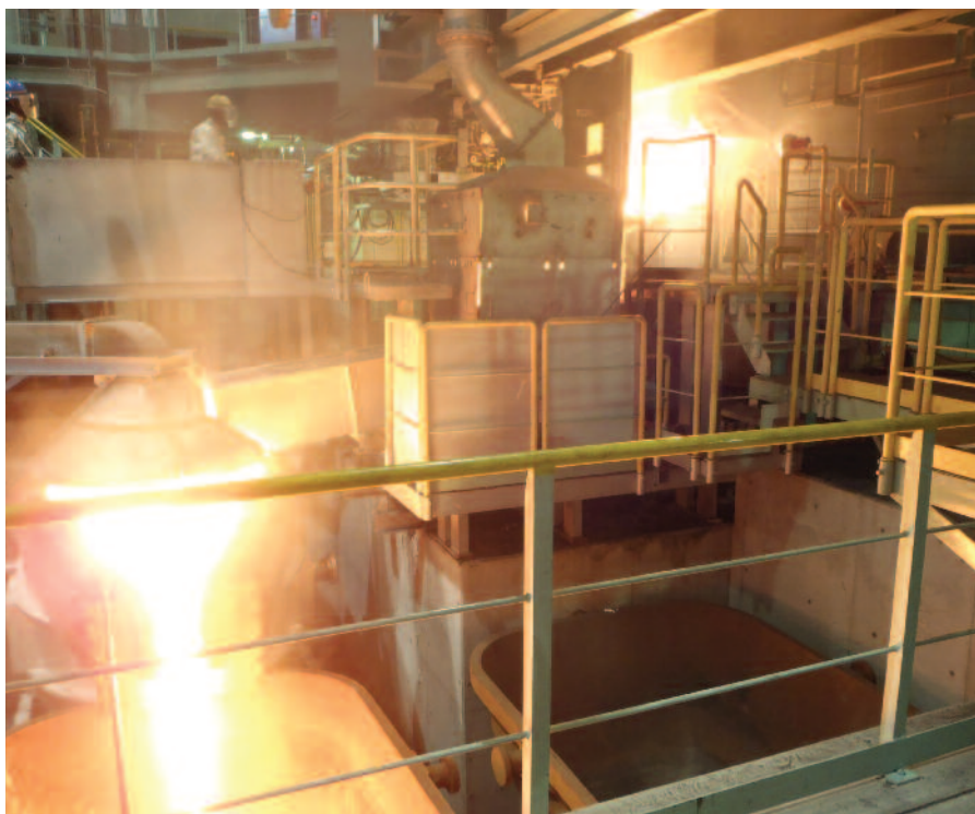
Tapping of the submerged arc furnace in the Hikari works.
