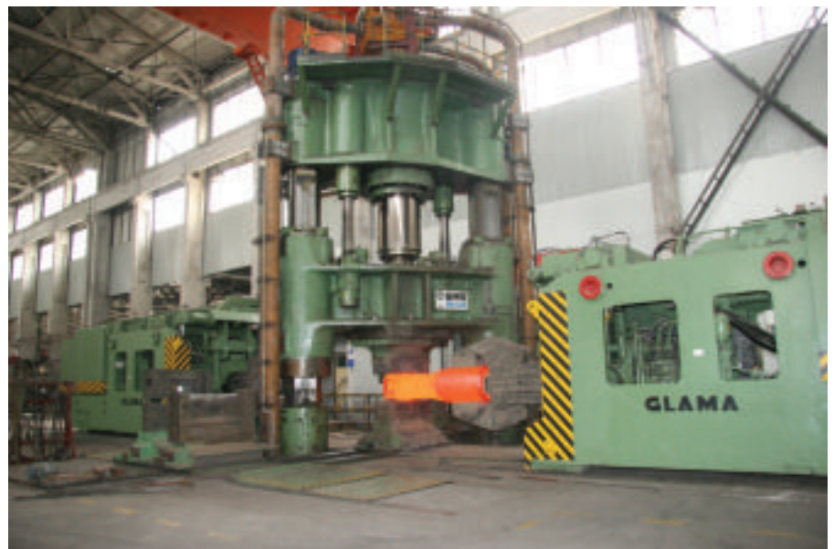
2500t fast speed forging press.
