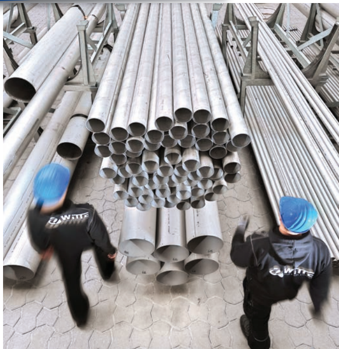
Seamless pipes being collected for an order. Before they are shipped out they will be sealed at their ends to protect the edges.
