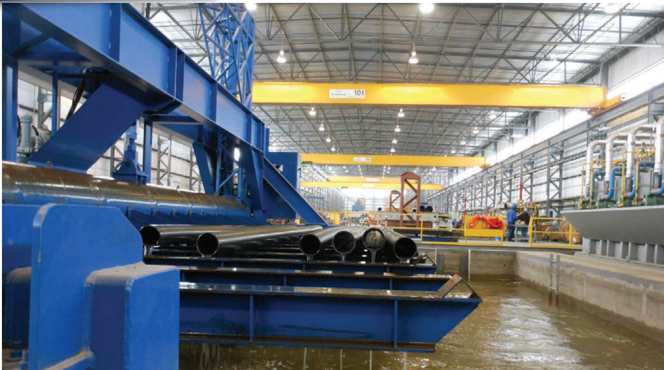
Pipes in the quenching process.
