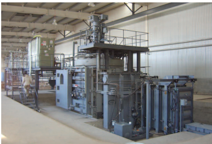
ESR furnace for nickel alloy products
