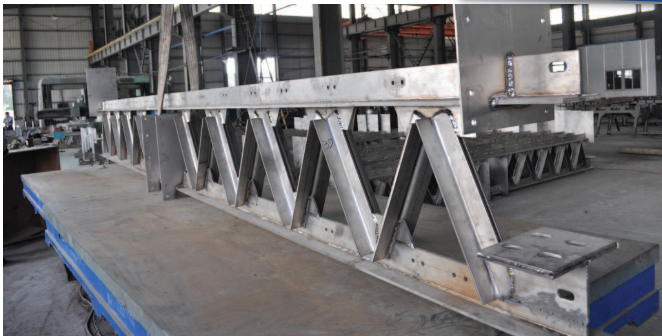
Titanium structure beam for PTA project
