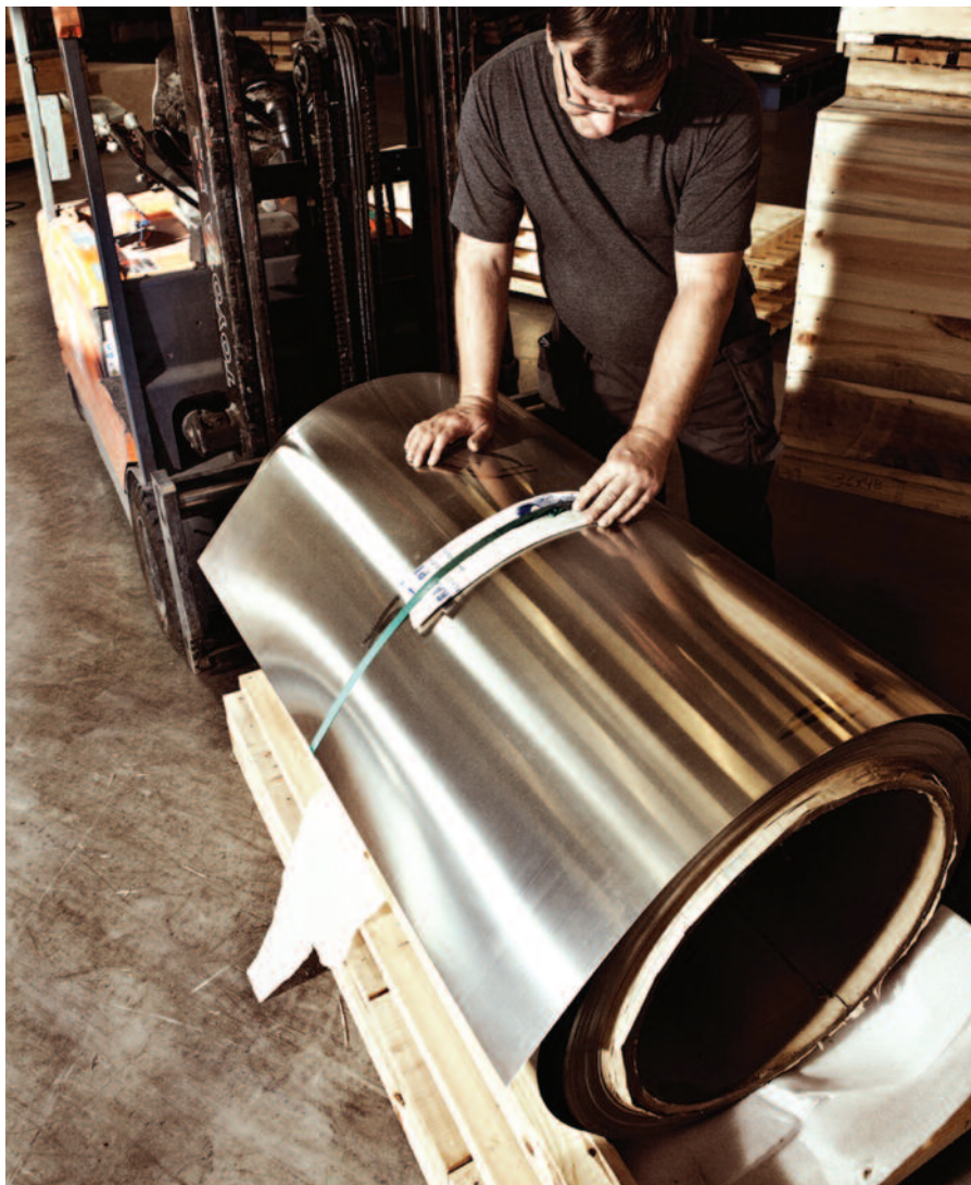
Coil is cut, slit or recoiled and put on a spool – all according to the customers needs. Harald Pihl offers all coils in custom sizes as part of their service.
