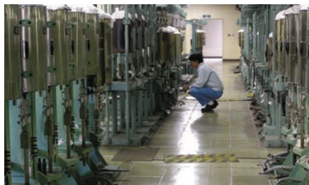
Creep test facilities in corporate R&D laboratory
