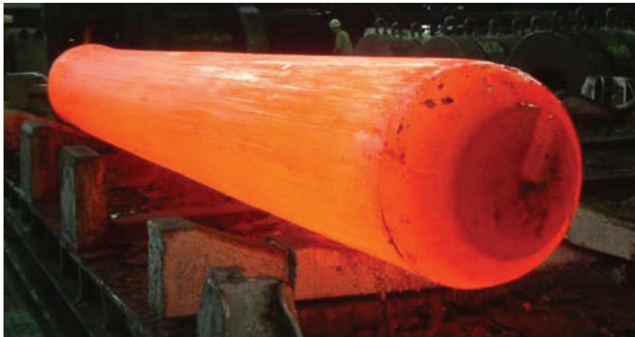
Large diameter thick wall pipe of HR6W (457mm in diameter with 60mm thickness)
