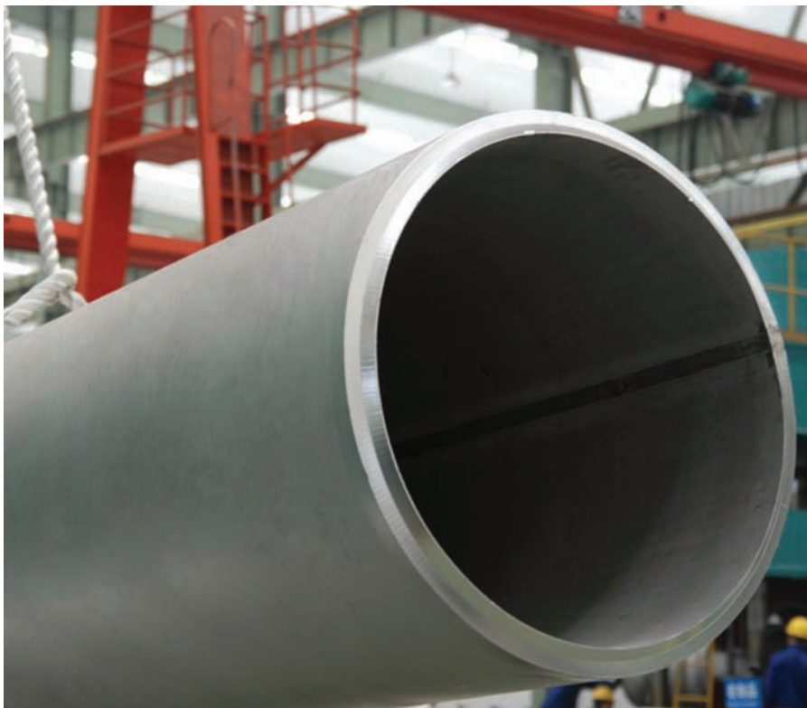
Welded pipe with heavy wall thickness.
