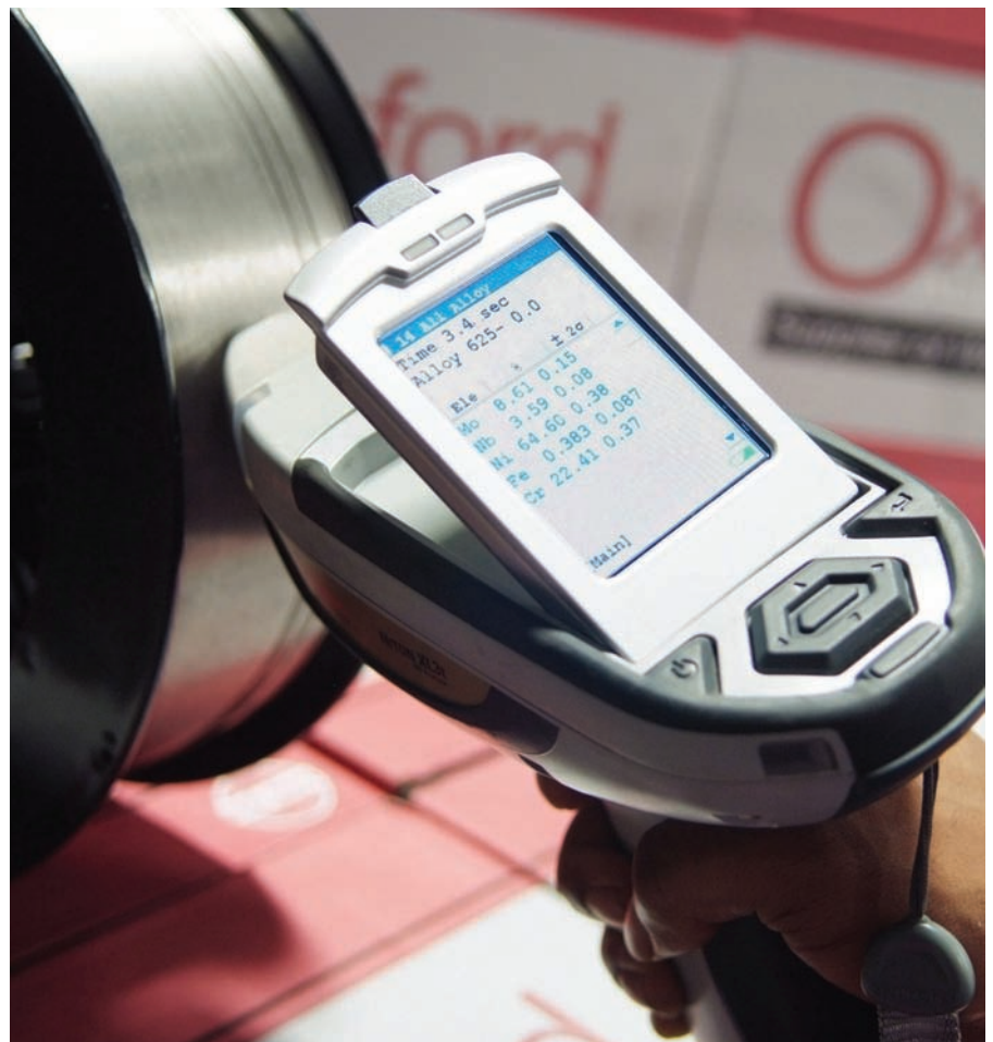
One of three camera enabled XRF instruments used to verify each products adherence to Oxford Alloys' stringent requirements.
