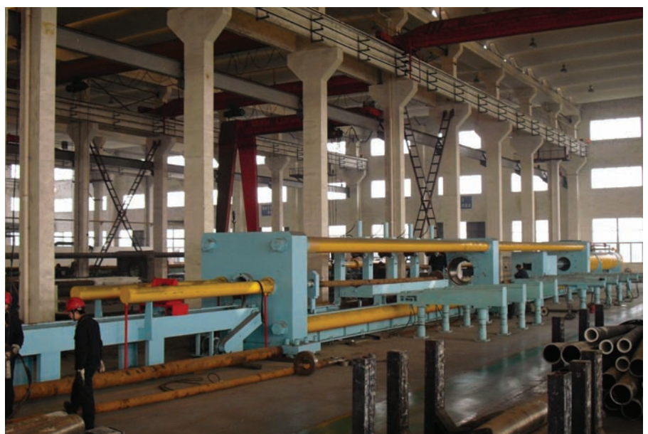
The 1000T hydraulic cold drawing machine at Wujin Stainless Steel could handle seamless stainless steel pipes with O.D. up to 1000mm.
