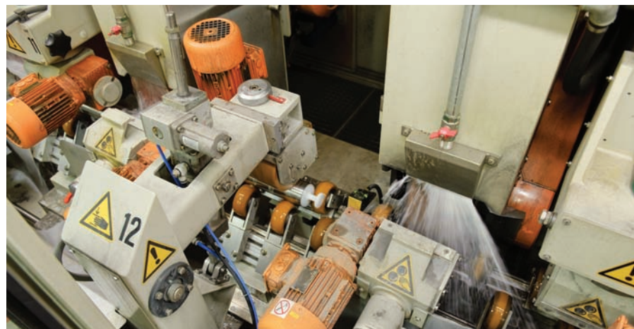
Mechanically polishing tube at RathGibson's Janesville facility.
