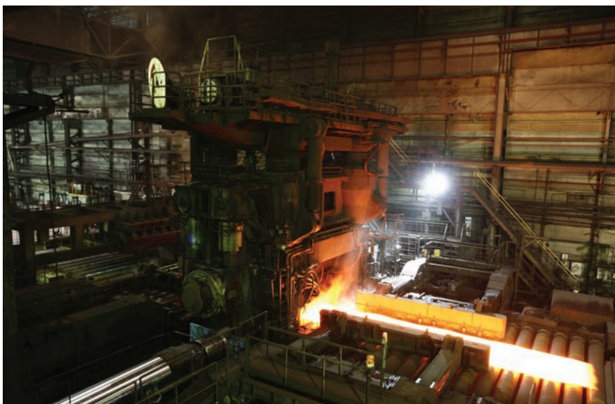
Finishing rolling mill at Yawata Works
