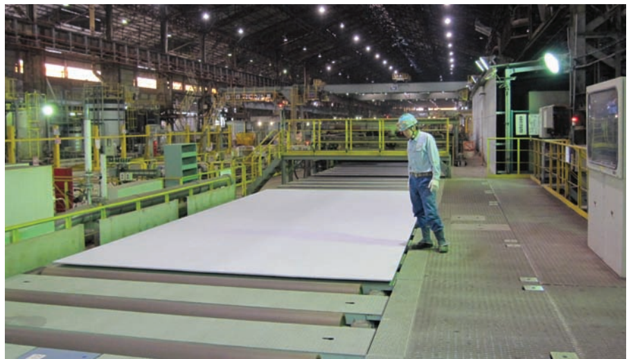
Wide plates with a maximum width of 4 metres are available.
