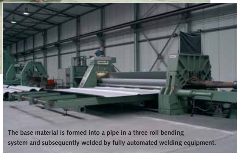
One of the continuous forming and welding process lines for welded stainless steel pipes manufactured from coil.
